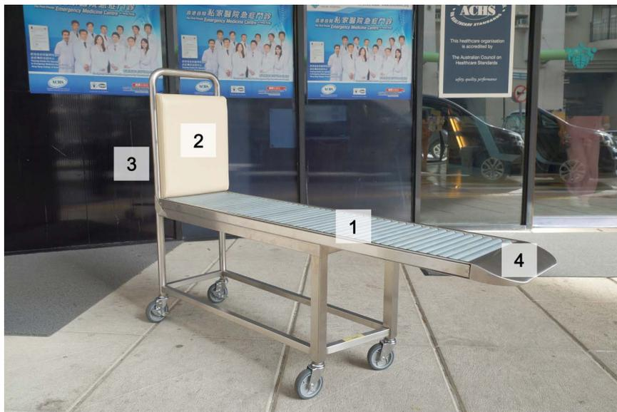
**Figure 1** The roller transfer plate. (A) The roller bearings on the platform are designed for easy sliding of patients. (B) Soft pad was added at the end of trolley to reduce the risk of injury. (C) The height of the trolley matches the height of the average seat to facilitate easy transfer of patients. (D) The frontal part of the trolley was a smooth ramp, which enabled patients to be moved onto the RTP with the least effort.
